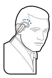
2 Holding the base of the headset, push it in and back towards your ear to allow the pivoting earpiece to bring the microphone close to your mouth. As the base of the headset moves backwards, you will feel soft clicks until the microphone rests close to your cheek.
