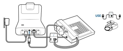
**2** While wearing your headset, slide the handset lifter arm under the handset until the lifter base touches the side of the phone.
