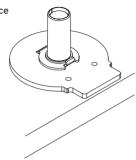
2 Attach spacer pad to C-bracket in required orientation
