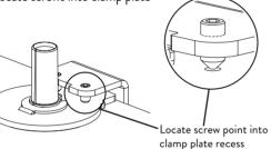
4 Tighten clamp screws
