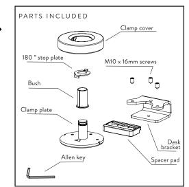
1 POSITION CLAMP PLATE ONTO WORK SURFACE
